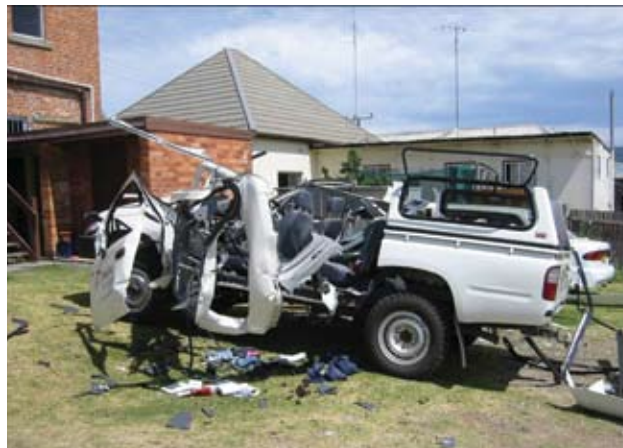
Aftermath of an explosion caused by a build-up of flammable gas in a vehicle
