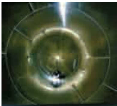
Figure 4 Welder TIG welding within a stainless steel vessel
